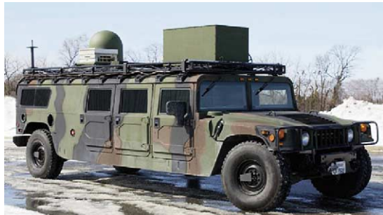
Fig. 2. Command and control combat vehicle with 2 kW fuel cell APU mounted on the roof.
